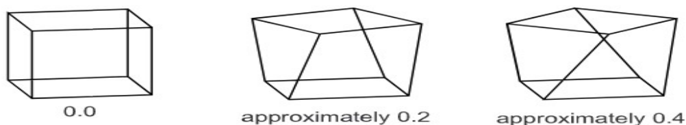
Figure: Bricks with various Warping Factors
